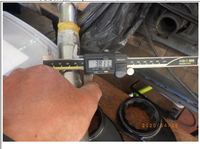
15 プロペラ側軸径⇒φ38.11 (1"1/2=38.1)
